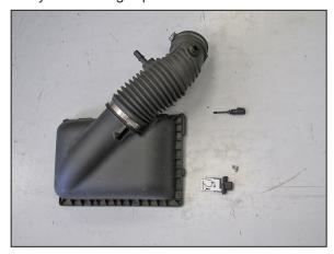
11. Remove the two screws securing the humidity sensor then remove the humidity sensor from the air filter housing. Remove the inlet air temperature sensor from the stock intake tube.
