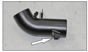
14. Install the humidity sensor into the K&N<sup>®</sup> intake tube and secure with the provided hardware.
