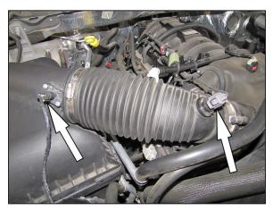
3. Disconnect the inlet air temperature sensor and humidity sensor electrical connections.
