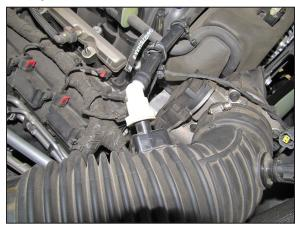
4. Depress the locking tab and then disconnect the crank case vent hose from the factory intake tube.
