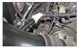
18. Connect the factory crankcase vent hose to the quick disconnect fitting on the K&N® intake tube.
