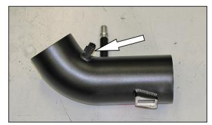
13. Remove the O-ring from the inlet air temperature sensor and then install the sensor into the grommet installed into the K&N® intake tube during the previous step.
