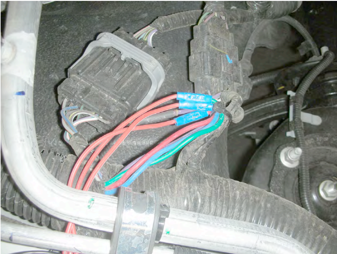
Engine compartment wiring connected to light harness.
