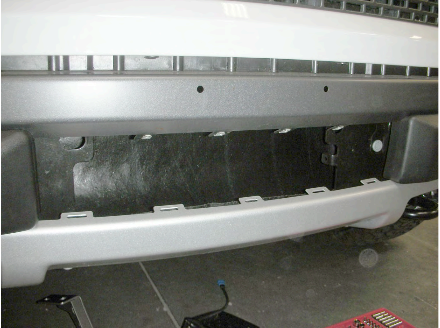
Lower grill removed.
