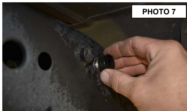
Spacer is used on driver rear only.
