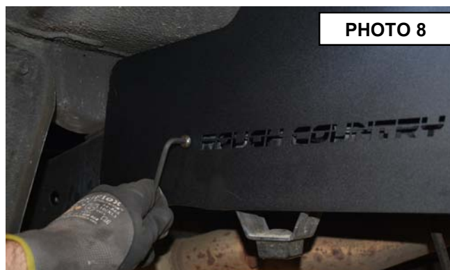
Tighten using a 3/16" Allen.
