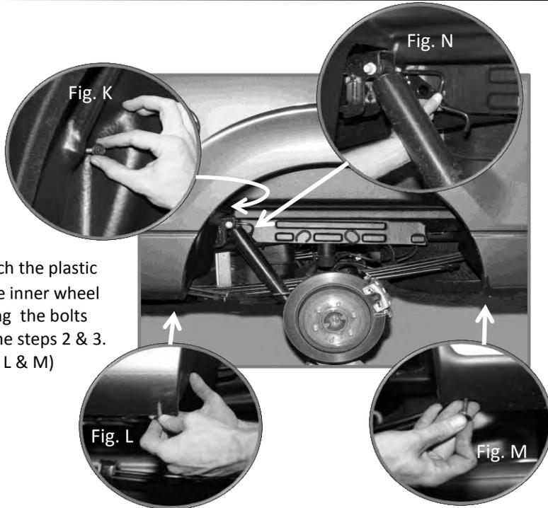
8. Re-install the plastic push pin that holds the gas exhaust hose (removed from step 5). Insert the push pin through the pre-drilled hole on the plastic protector and the hole on the chassis frame. (see fig. N)
