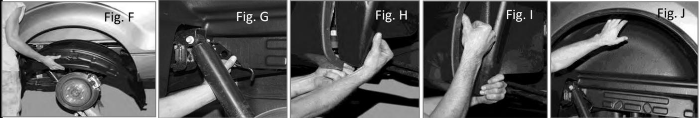
6. **a)** Place the Rear Wheel Well Inner Liner marked as "DS" (Driver side) on the inner panel of the wheel house. Make sure to go up & over the shock and shock mounting bracket first. (See Fig. F & G)
