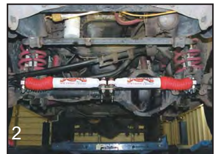
Both brackets mount in the same direction. (see step 6 above)
