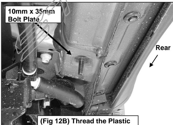
(Fig 12B) Thread the Plastic Retainer onto the Bolt Plate
