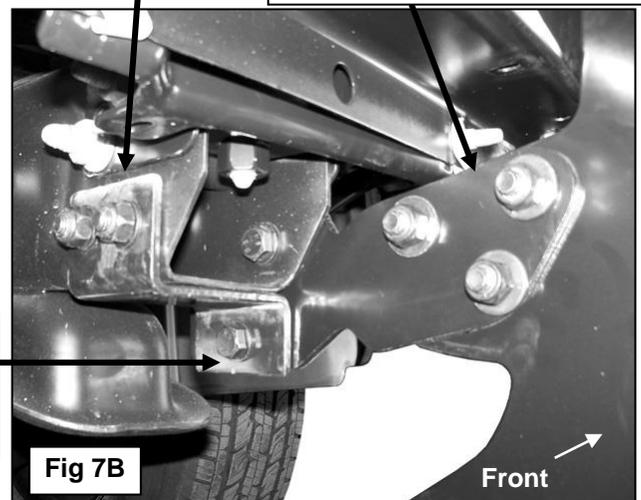
**Passenger Side Mounting Bracket Installation Pictured**
