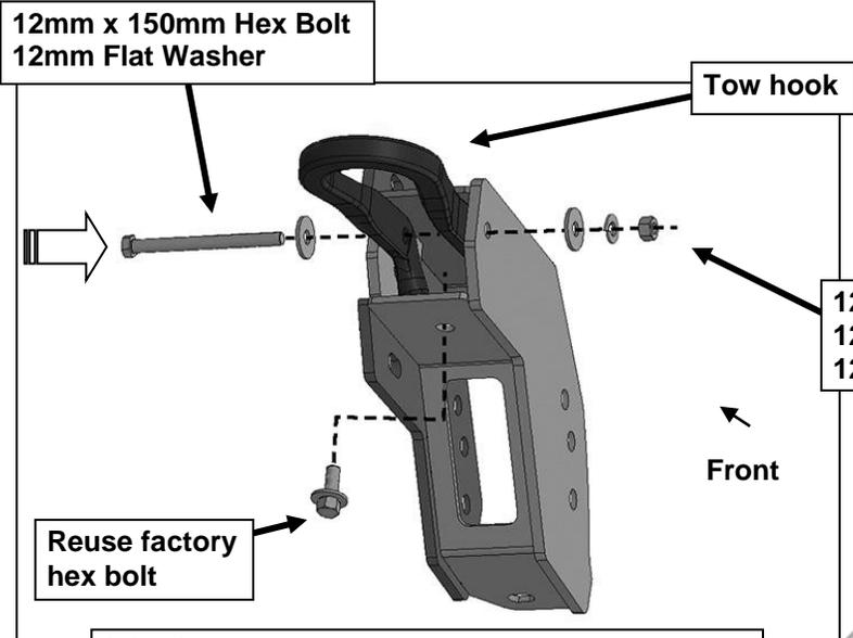
(Fig 3) Attach the tow hook to the passenger side Frame Bracket. **IMPORTANT:** Insert 12mm x 150mm Long Hex Bolt with (1) 12mm Flat Washer from outside to inside only
