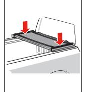
Unfold the bed cover (A) fully and adjust position over the truck bed for proper front (cab) and rear (tailgate) alignment. When positioned front and back, the tailgate seal should contact the tailgate with the first two fins.
