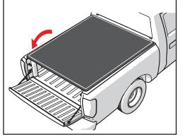
Align the latch with the tailgate striker bracket (C). Push down on the cover while tightening the Torx screws (B) with the supplied T-27 wrench.
