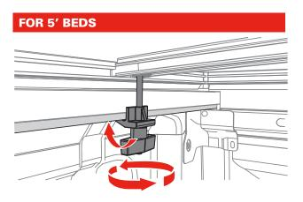
Hook the cab clamp under the truck bed rail metal flange. Tighten the knob until the jaw makes contact, then turn an additional two turns. Repeat on the opposite side of the truck bed.
