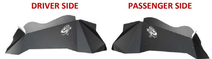
Flex and manipulate your new inner fender to work it into the fender well and around your tire. Work the inner fender until you have snapped it into place around all the Jeep fender edges and frame.
