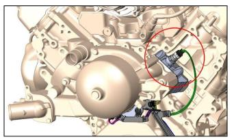
Torque temperature sensor to 15 ft/lb
