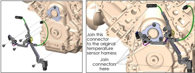
NOTE: Torque bolts M6 bolts to 11 Ft/lbs
