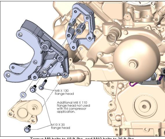
If installing an R4 compressor and bracket, additional step are described below.
