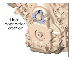
2. Install supplied harness assembly as shown. Make sure no wiring is pinched between engine and harness bracket. Reinstall the four harness bolts. Join the five connectors shown and engage red connector locks.
