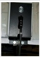
Continue along the side of the vehicle to the 5th mounting bracket repeat steps 3, 4 for the lower mounting holes.
