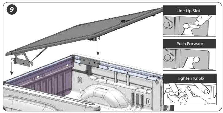
9. With some assistance place the cover onto the front mounting brackets. . Line the open slot up in the hinge with the pin on the mounting bracket. Push the cover forward to lock it into place. Tighten knob until it stops, it may be necessary to push the hinge up tight to the mounting bracket to help the threads engage, be careful not to cross thread and strip the bracket.
