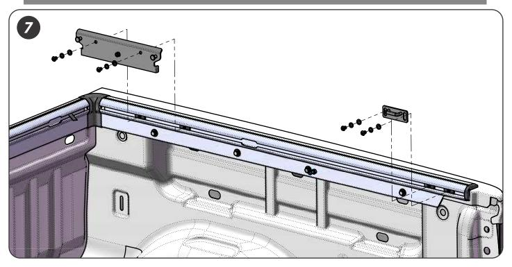
7. Slide four (4) M8 t nuts into each tango side rail track. Using the M8 bolts, flat washers and lock washers attach the front brackets and the striker brackets according to the measurements below.
