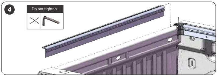
4. Slide front rail assembly by inserting L bracket into T-slot, do not tighten set screws.
