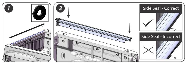
1. Clean the bulkhead and install the bulk head seal.
