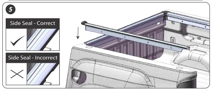
5. Slide the left rail assembly in place by inserting the L bracket in to the T-slot, do not tighten Note: Lift up on the front rail assembly to create enough room to insert the L bracket into the T-slot. Note: Be sure side rubber is not pinched under rail assembly.
