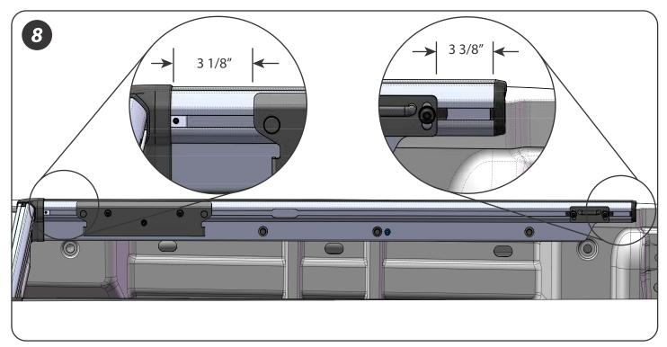
8. Position the front mounting brackets 3 1/8" from the plastic corner piece of the Tango Track. Position the rear striker brackets 3 3/8" from the rear of the extrusion.
