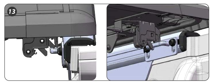
13. Close the cover and check that the latches properly engage to the striker bracket. To adjust up or down, loosen the bolts on the striker bracket. To adjust side to side loosen the nuts on the rotary latch. The cover will latch or unlatch with the emergency release with the lock unlocked or locked.
