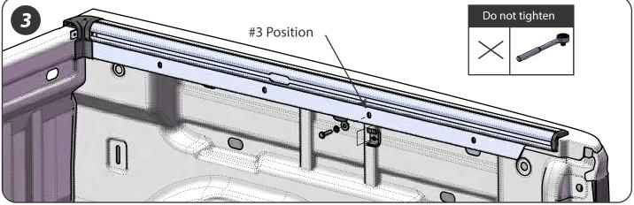
3. Install one clamp in the #3 position, do not tighten completely.
