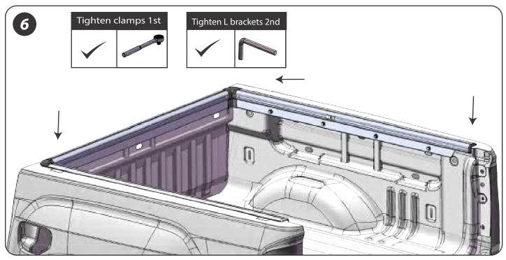
6. Push Tango system towards bulkhead, install all remaining clamps and tighten.
