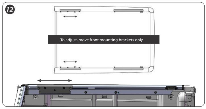
12. With your cover closed, take a quick inspection to make sure that the cover is sitting square to the Tango Track. To adjust the cover front to back evenly, move both of the front mounting brackets forward or rearward accordingly. To adjust to one side or the other, move the front mounting brackets forward or rearward independently.
