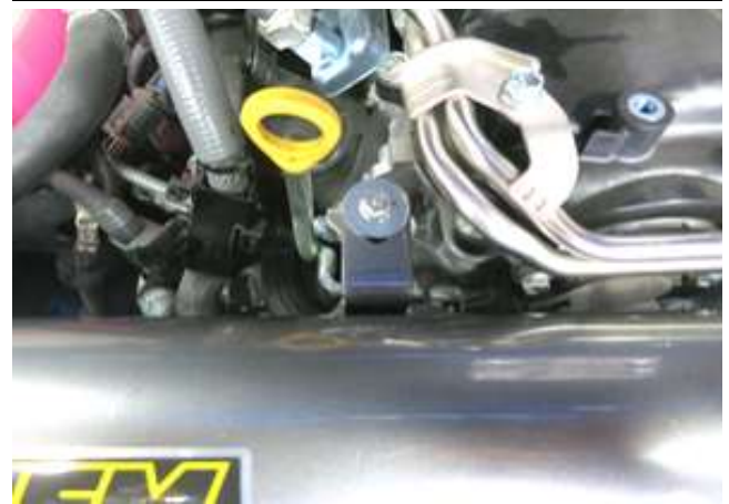
j. Adjust the intake pipe for best fitment, making sure it isn't hitting any surrounding components. Then, fasten the mounting bracket to the soft mount with the supplied fender washer and M6 flanged nut.
