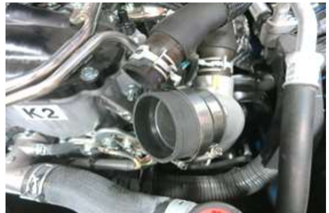
h. Place the tapered, reinforced coupler onto the turbo inlet pipe. Make sure the smaller diameter end is on the turbo inlet side. Then, place the 2 small hose clamps onto the coupler. Leave the hose clamp on the intake pipe side loose. Tighten the hose clamp on the turbo inlet side to 30 in-lbs.
