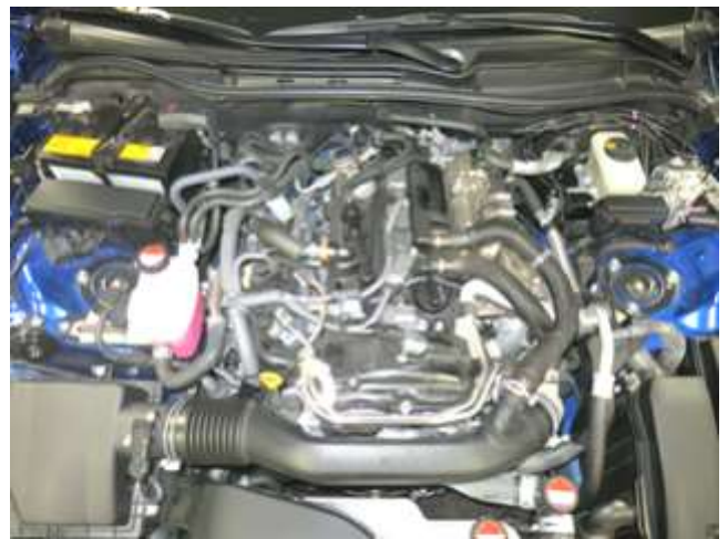
b. Carefully pull up on the engine cover and remove it.
