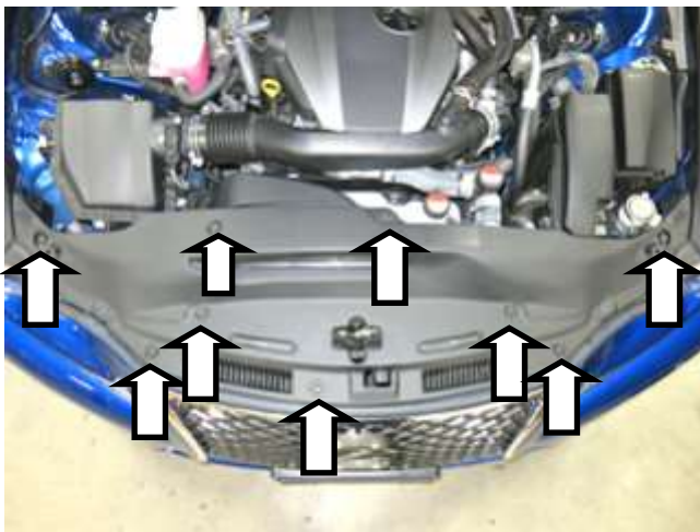
a. Remove the 9 push clips that hold the radiator shroud in place.
