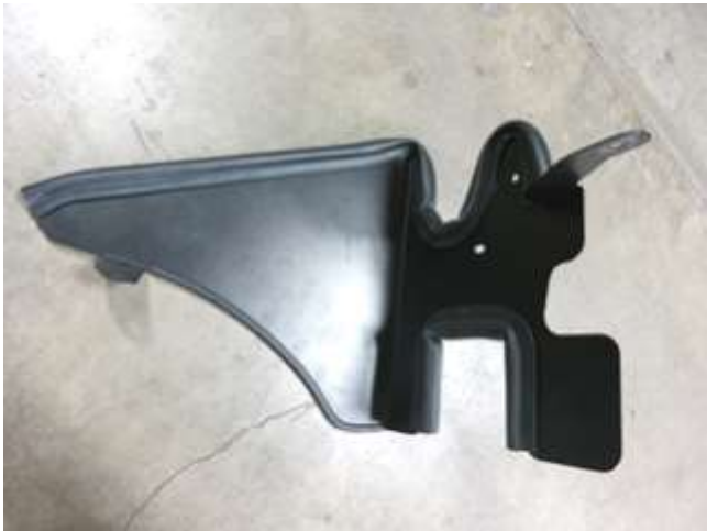
d. Apply the supplied edge trim to the heat shield, as shown above.
