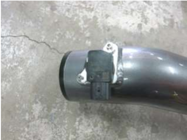
b. Attach the MAF sensor to the intake pipe using the 2 provided M4 bolts.
