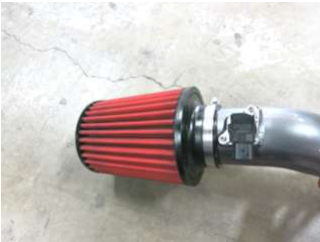
c. Attach the air filter, with the large hose clamp, to the intake pipe. Use an 8mm socket and ratchet, or a flat head screw driver, to tighten the hose clamp to 30 in-lbs.
