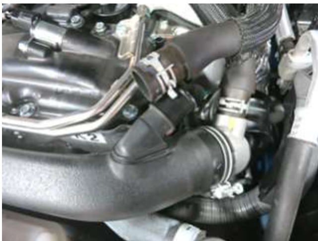
c. Use pliers to relieve tension on the hose clamp and then pull the breather hose off of the stock intake tube port.
