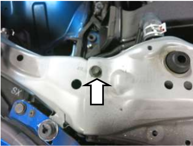
e. Use a 10mm socket and ratchet to remove the M6 bolt, shown above.
