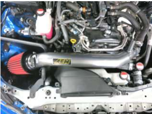
i. Insert the assembled AEM intake pipe into the turbo inlet pipe coupler. Make sure the mounting bracket on the intake pipe aligns with the soft mount.
