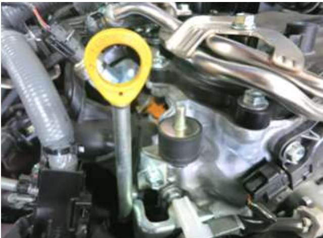
g. Screw the supplied soft mount to the engine bracket.
