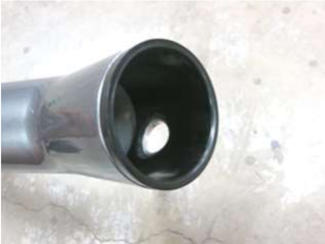
a. Insert the venturi into the AEM intake pipe. Make sure the cutout in the venturi aligns with the cutout in the intake pipe.
