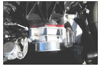
**5.** Vehicles equipped with plastic intake manifolds have an O ring pressed into the throttle body mounting surface. On these applications only a single gasket is to be used between the spacer and the throttle body. Discard the second gasket.
