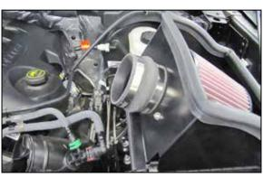
13. Install the provided coupling hose (08699) onto the filter adapter and secure with the provided hose clamp.
