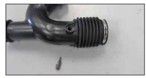
17. Unlock the inlet air temperature sensor and
