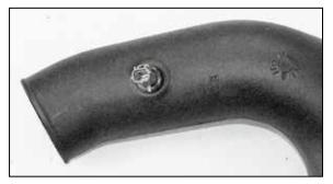
18. Remove the O-Ring from the inlet air temperature sensor and then install it into the grommet installed into the K&N<sup>®</sup> intake tube. . NOTE: The inlet air temperature sensor is very fragile, be careful while installing the sensor so as not to break it. NOT LEGAL FOR SALE OR USE ON ANY POLLUTION CONTROLLED MOTOR VEHICLE IN CALIFORNIA OR STATES ADOPTING CALIFORNIA EMISSION PROCEDURES.
