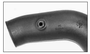
16. Install the provided grommet into the K&N<sup>®</sup> intake tube as shown.
