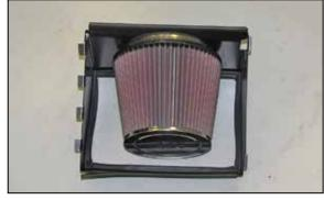
11. Install the K&N<sup>®</sup> air filter onto the filter adapter
