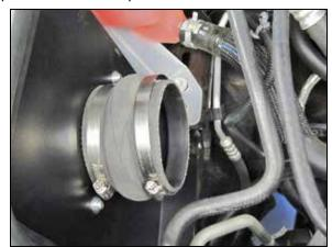
14. Install the coupling hose (08418) to the filter adapter and secure with the provided hose clamp.
