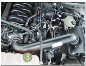
14. Install the K&N® intake into the coupling hose at the filter adapter and then into the hose at the throttle body, adjust the tube for best fit and then secure with the provided hose clamps.
