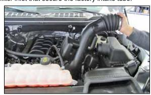
4. Unhook the coolant line from the intake tube and then remove the intake tube from the vehicle.
