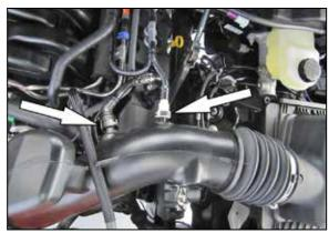
2. Disconnect the EVAP vent connection and crank case vent connection.
