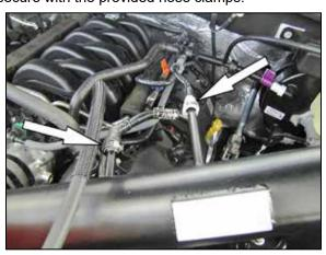
15. Connect the factory EVAP and Crank case vent
