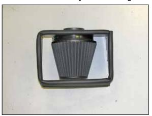
10. Install the air filter onto the filter adapter and secure with the provided hose clamp.
