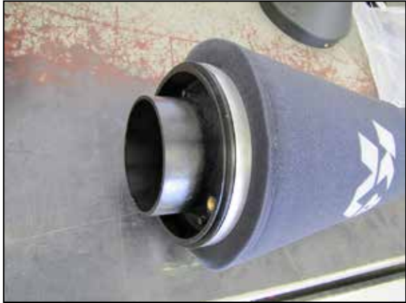
2. Install the radius filter adapter into the air filter and secure with the provided hose clamp.
