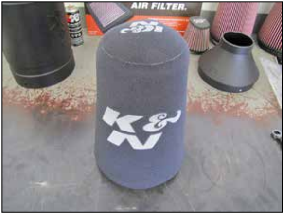
1. Install the Extreme Duty Foam Wrap onto the filter.
