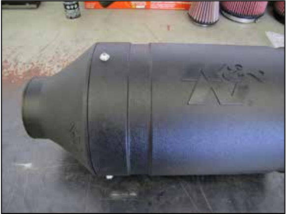
6. Install the canister lid onto the canister and secure with the provided hardware.
