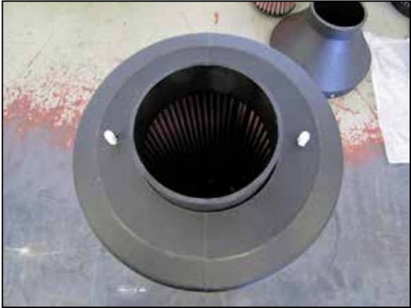
4. Install the filter assembly into the canister so that the studs protrude out of the holes.
