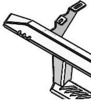
**Note:** Larger bracket attaches towards the front of the channel
