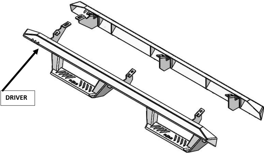
**Step 2:** Install three rocker panel brackets to the attachments points located on the backside of the channel using the supplied 3/8" x 3/4" carriage bolts and 3/8" flanged nuts. Leave finger tight for now.
