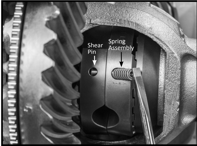
Figure 7: Install spring assemblies in holes
