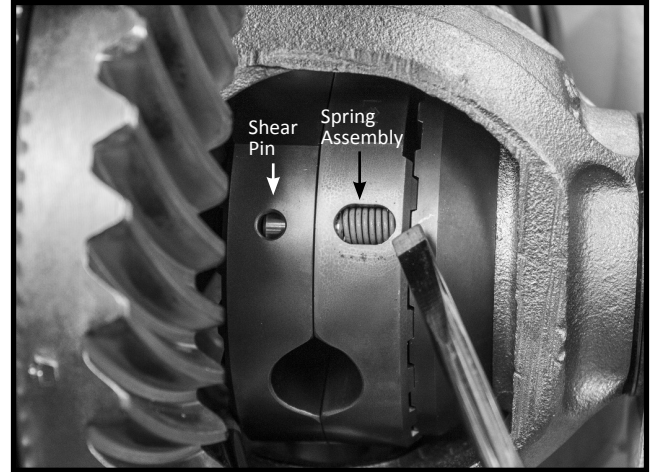
Figure 8: Snap spring assembly into hole
