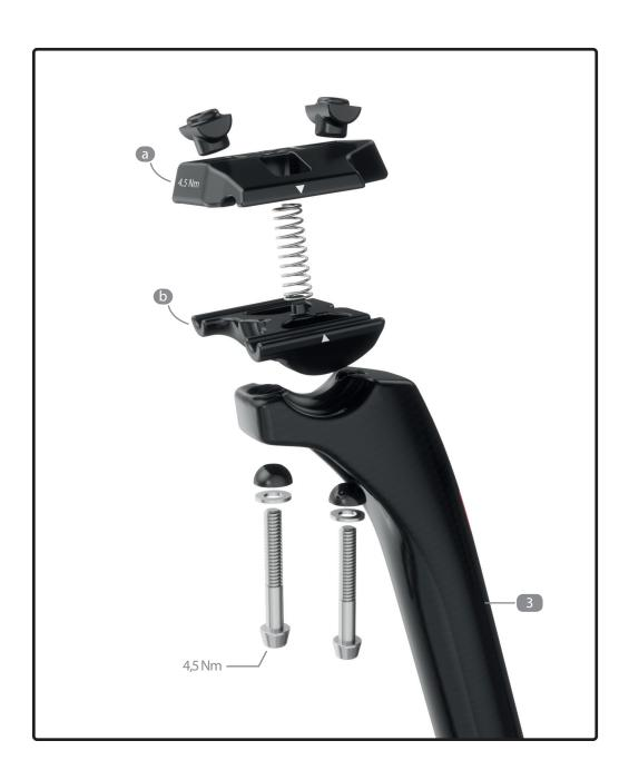
The seat post (3) is supplied fully assembled. It's equipped with a spring-loaded head for easy installation of the saddle.
