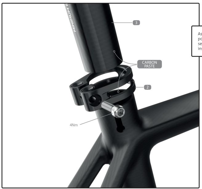
Assemble the seat post collar (2) with the seat post (3). Apply carbon paste inside the frame's seat tube and on the seat post where it inserts inside the frame. Tighten the bolt at 4 Nm.
