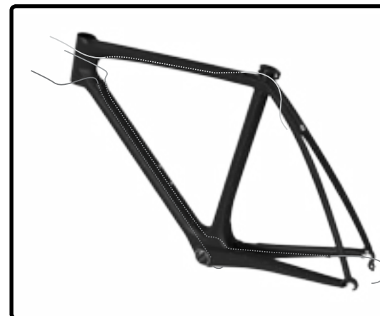
3. Cable housing installation
