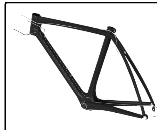
3. Cable housing installation
