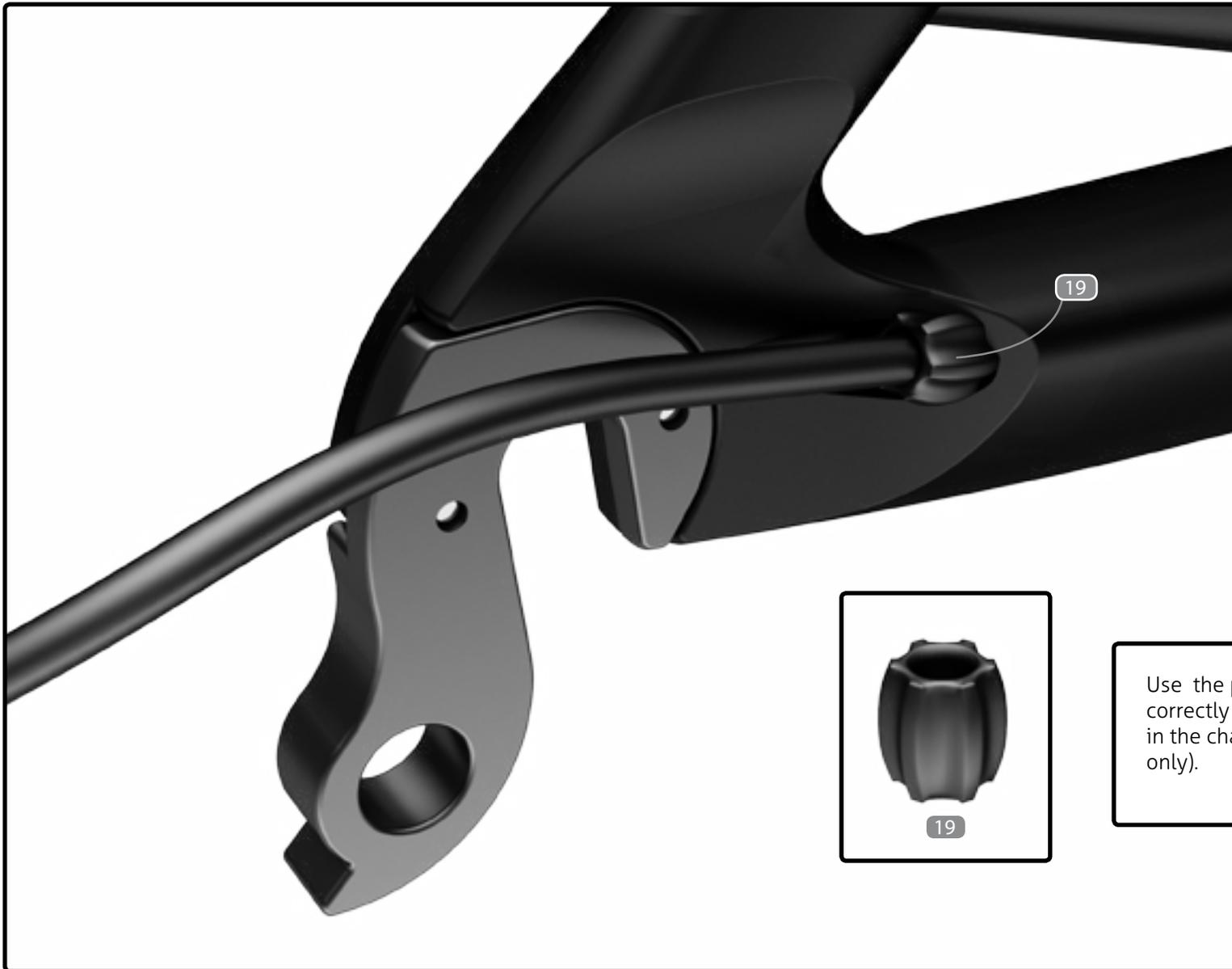
Use the provided grommet (19) to correctly set the rear derailleur cable in the chainstay (mechanical drive train only).
