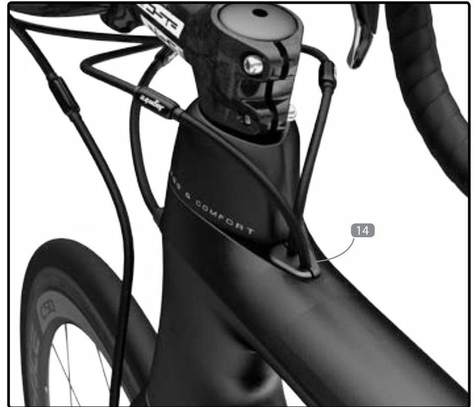
Use the proper grommet on the top tube to fix the cable correctly (depending if you use electronic shifting or mechanical drive-train).
