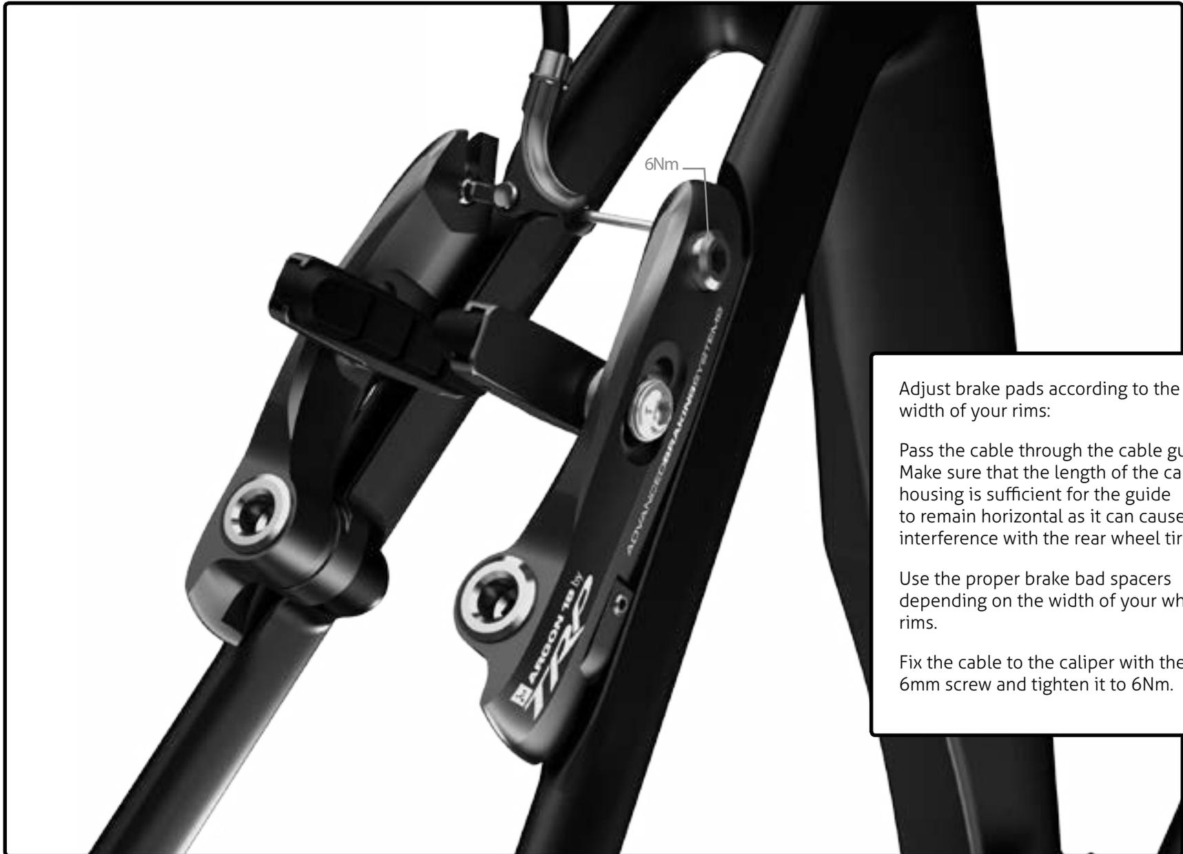
Adjust brake pads according to the width of your rims:
