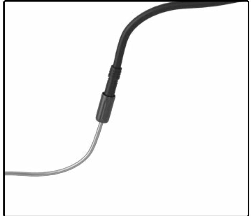
The Di2 cable routing can be achieved easily using this simple trick: use a brake cable and a metal cable end to fix the Di2 cable. For more information on Shimano Di2 electronic system installation, go to : <http://si.shimano.com>.
