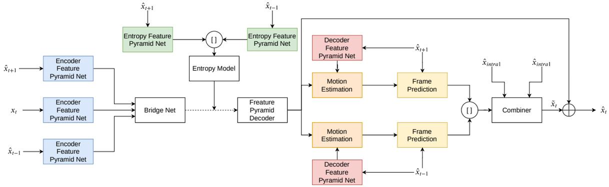
Figure 2. Architecture of the inter-frame codec
