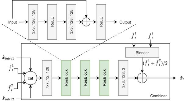
Figure 4. The Combiner, part of the inter-frame decoder.
