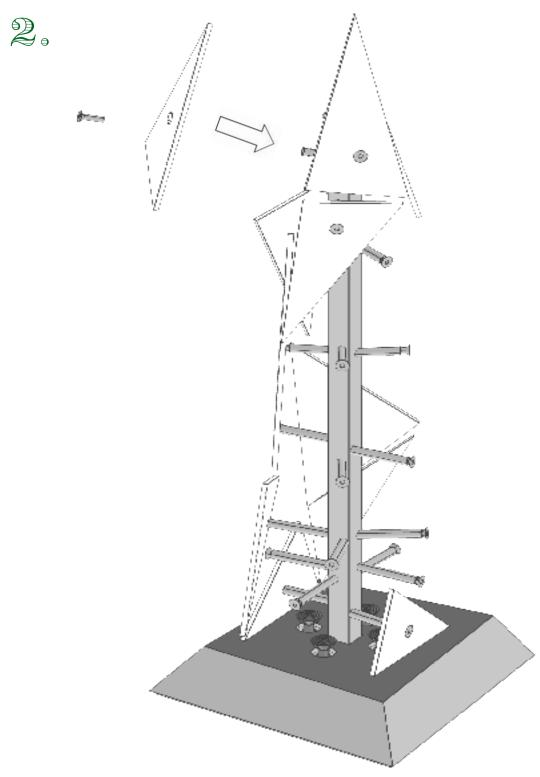
SCREW THE GLASS TRIANGLES BY MATCHING THE NUMBER OF THE TRIANGLE WITH THE NUMBER OF THE STEEL BUSHING. THE OPERATION MUST BE CARRIED OUT VERY CAREFULLY NOT TO OVERTIGHTEN THE SCREW, AVOIDING TO BREAK THE GLASS.
