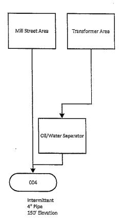
Maximum non contact cooling water flow = 0.7 MGD
