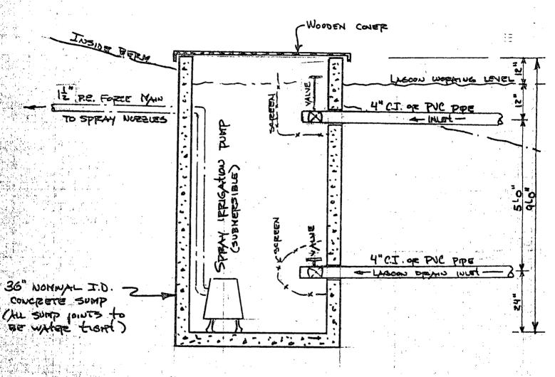
Note: Upper 4" with to extend approx. 18' into haccord of to be supported 12" began notified upper upter level Both ends of upper with to be appeared (HAV. OPENING SIZE 1/16") to prevent souds from external surp.
