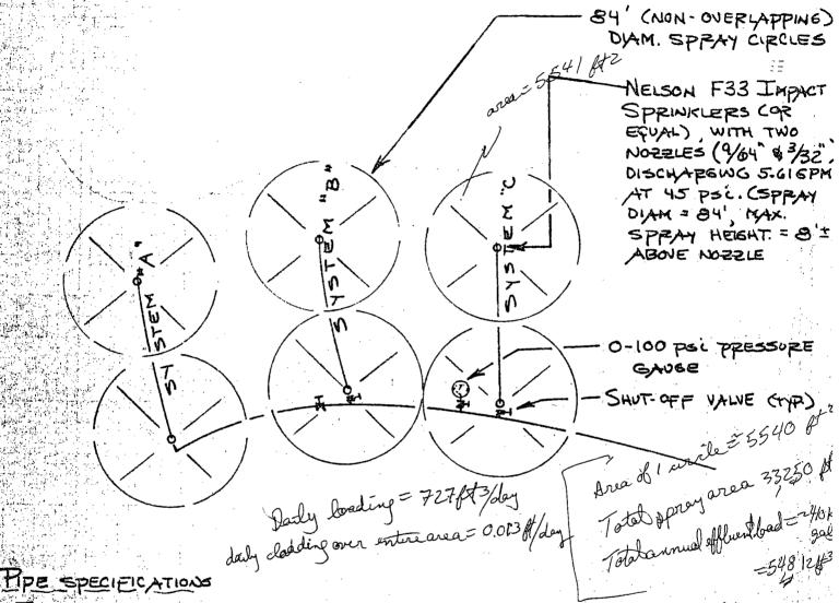
IPPRIGATION PIPING SHALL BE 100 PS'L BLACK POLYETHYLENE PIPE, 12" DIAM EXCEPT THAT I" DIAM MAY BE USED ON ANY LATERAL WITH ONLY (1) SPRINKLER.
