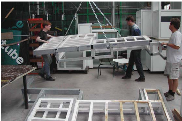
FIG. 64 Assembly sandwich walls
