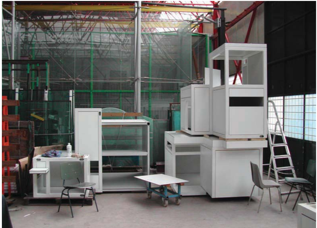
FIG. 66 Modulaire units ready of total assembly in Octatube laboratory
