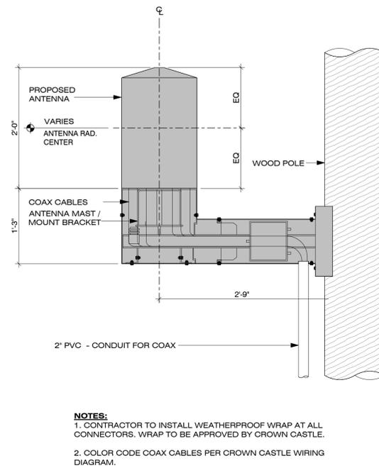
POLE-TOP EXTENSION / ANTENNA DETAIL SCALE: 1"=1'-0" 20
