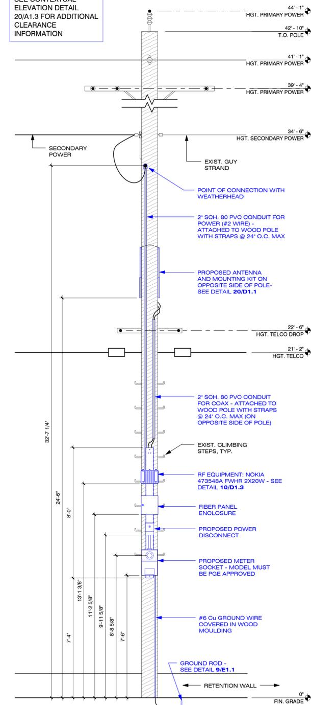
POLE ELEVATION - PROPOSED (LOOKING SOUTH) SCALE: 3/8" = 1'-0" 20
