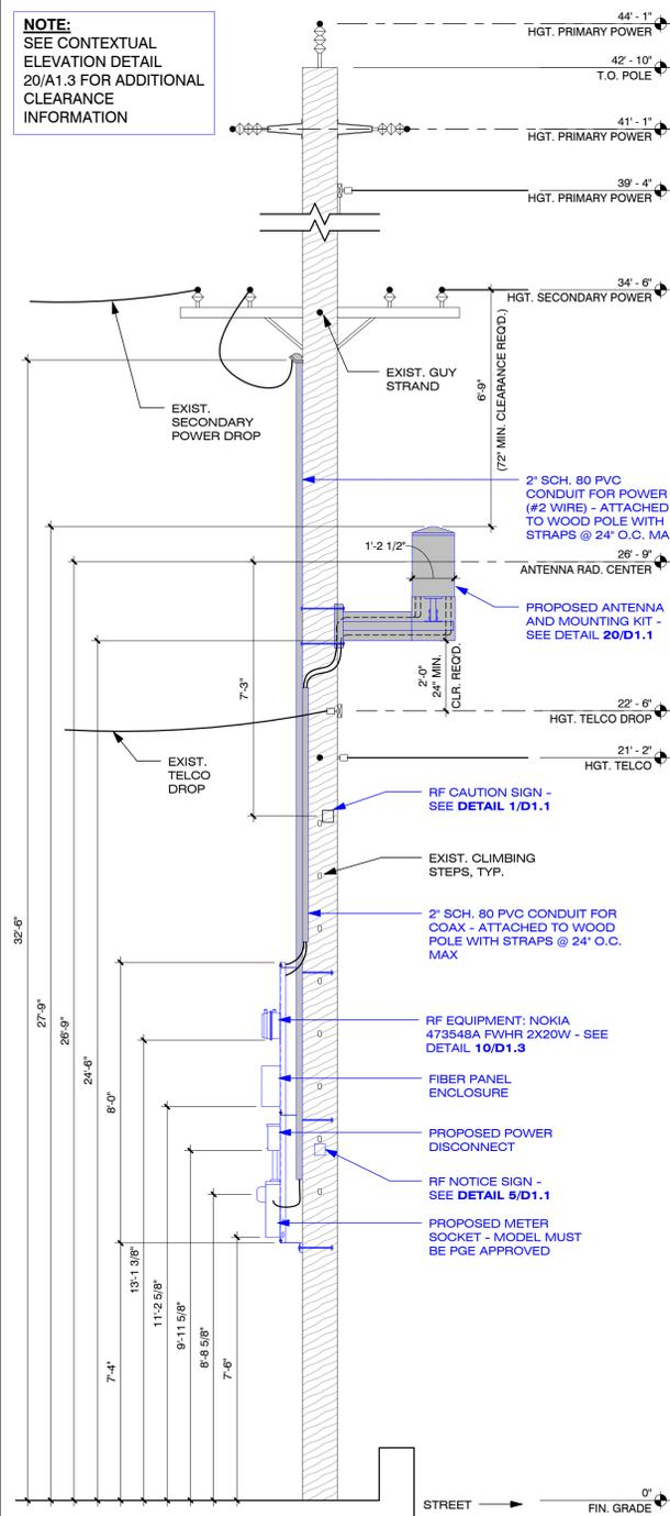
POLE ELEVATION - PROPOSED (LOOKING EAST) SCALE: 3/8" = 1'-0" 16
