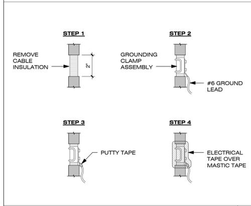
COAXIAL CABLE GROUNDING SCALE:N.T.S. 2
