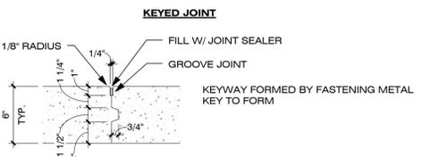
CONCRETE JOINT DETAILS SCALE: N.T.S. 10
