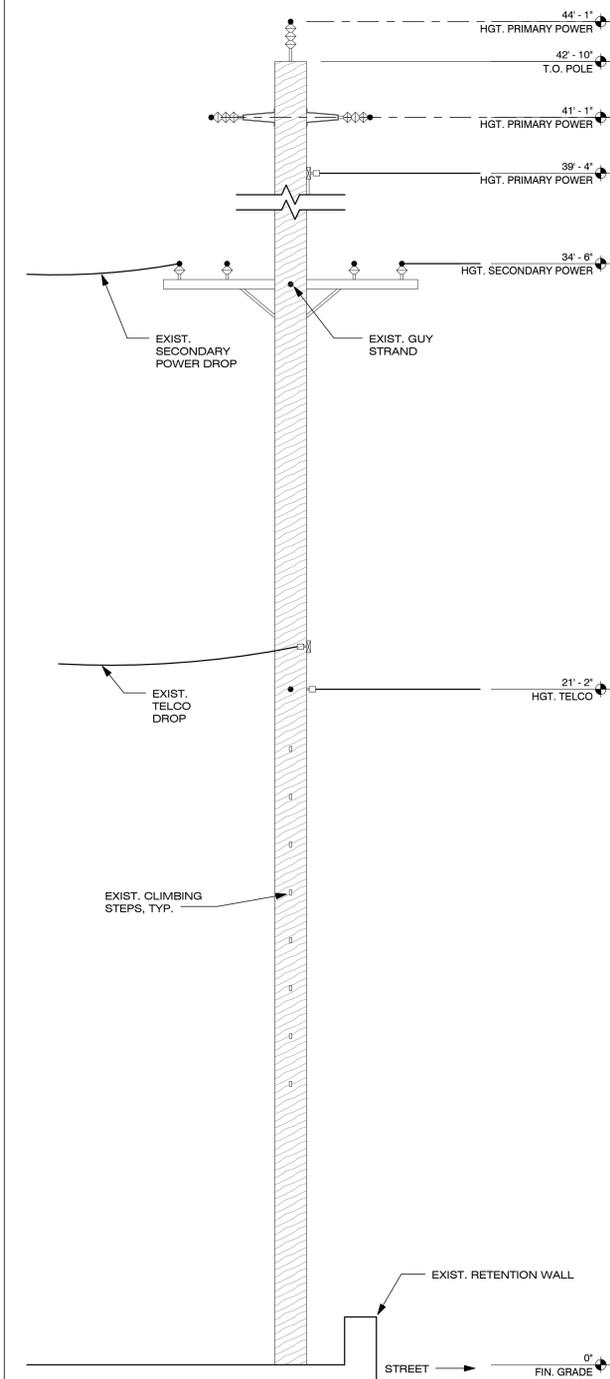
POLE ELEVATION - EXISTING (LOOKING EAST) SCALE: 3/8" = 1'-0" 16
