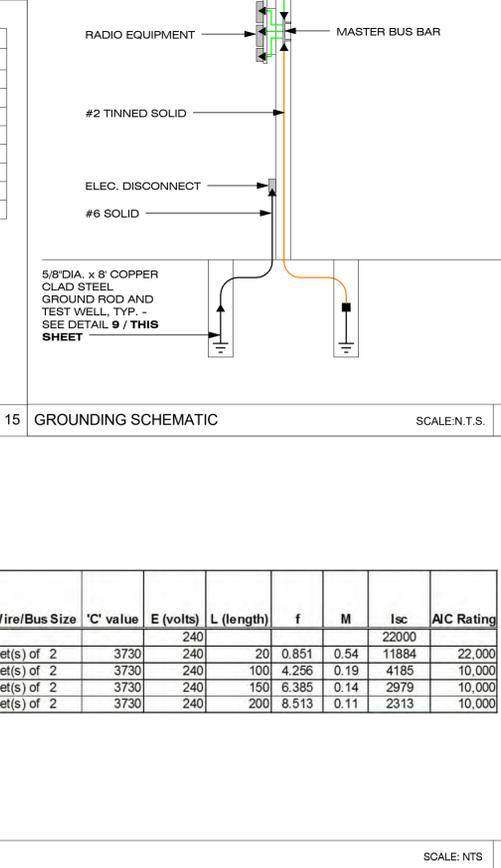
GROUNDING SCHEMATIC SCALE:N.T.S. 19
