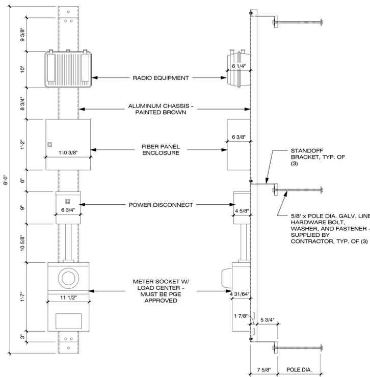
EQUIPMENT MOUNTING CHASSIS DETAIL SCALE: 1"=1'-0" 12
