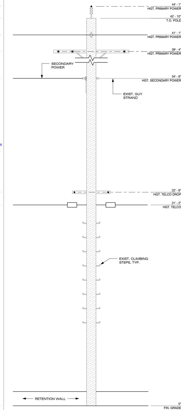
POLE ELEVATION - EXISTING (LOOKING SOUTH) SCALE: 3/8" = 1'-0" 16
