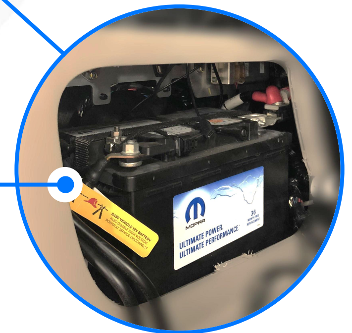
Base vehicle 12 V battery (trim panel is removed on Waymo Pacificas)
