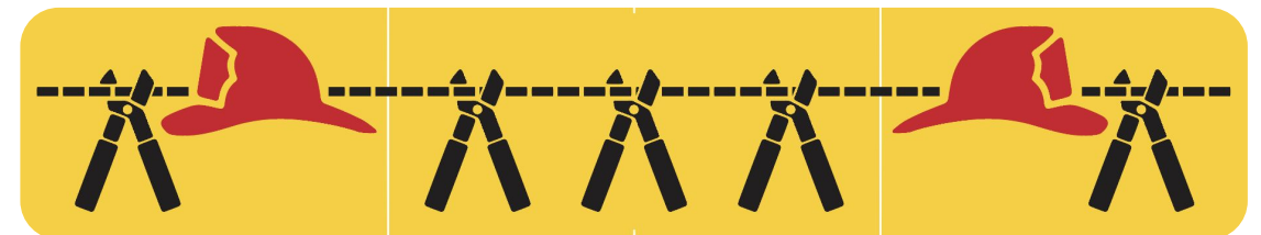
First responder cable cut loop tag in vehicle
