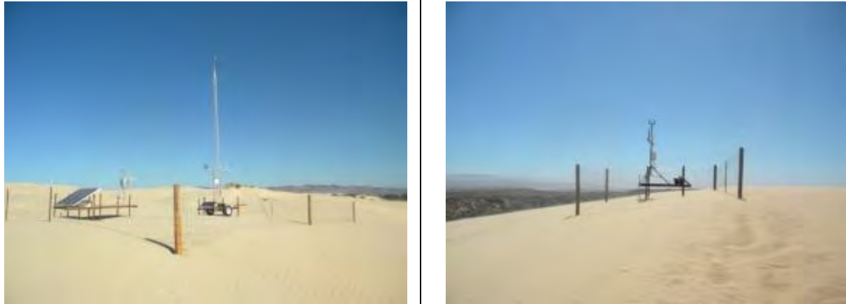
Figure 6-12. Left: Temporary monitoring site with E-BAM, solar panels, and 10-meter lattice tower (approximately 0.1 acre). Right: Temporary monitoring site without E-BAM and 10-meter tower (approximately 0.05 acres).
