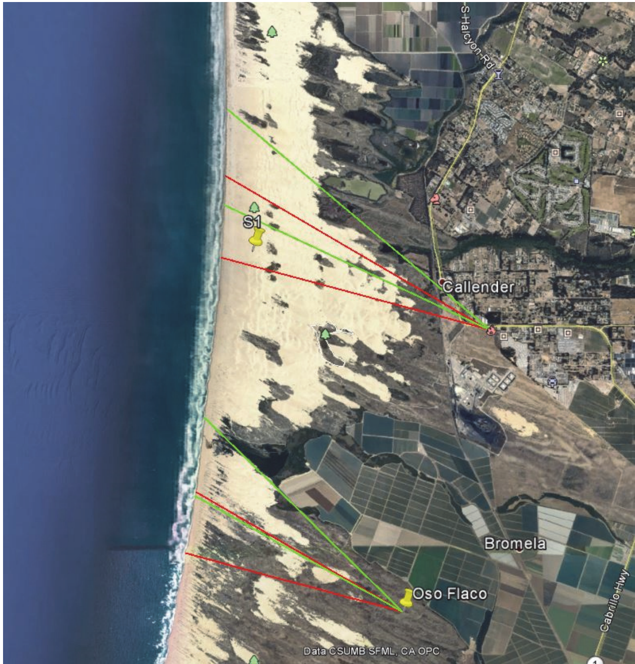
The 285-300 degree arcs used by CGS are shown in red. The 299-314 arc for Oso is shown in green, as is the 295-310 degree arc representing the most frequent wind directions recorded at CDF during high wind/PM events.
