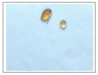
Filter jcpft138 with evidence of contamination (X60)
