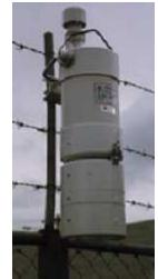
Figure 2. PM2.5 Mini-Vol Sample Example
