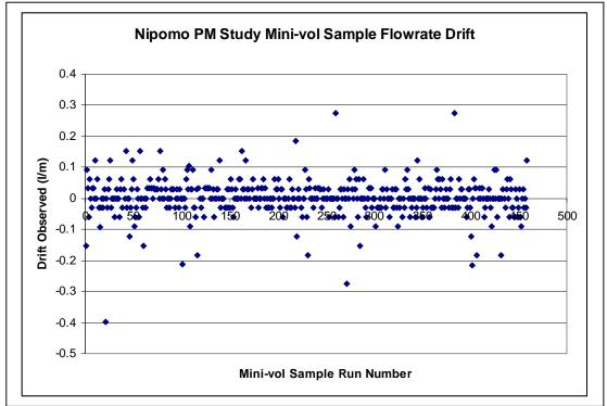
Figure A-4. PM2.5 Sampler Flowrate Drift
