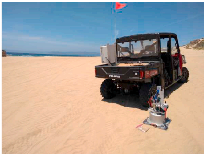
Fig. 2. The PI-SWERL at a test location in the riding area of the ODSVRA.
