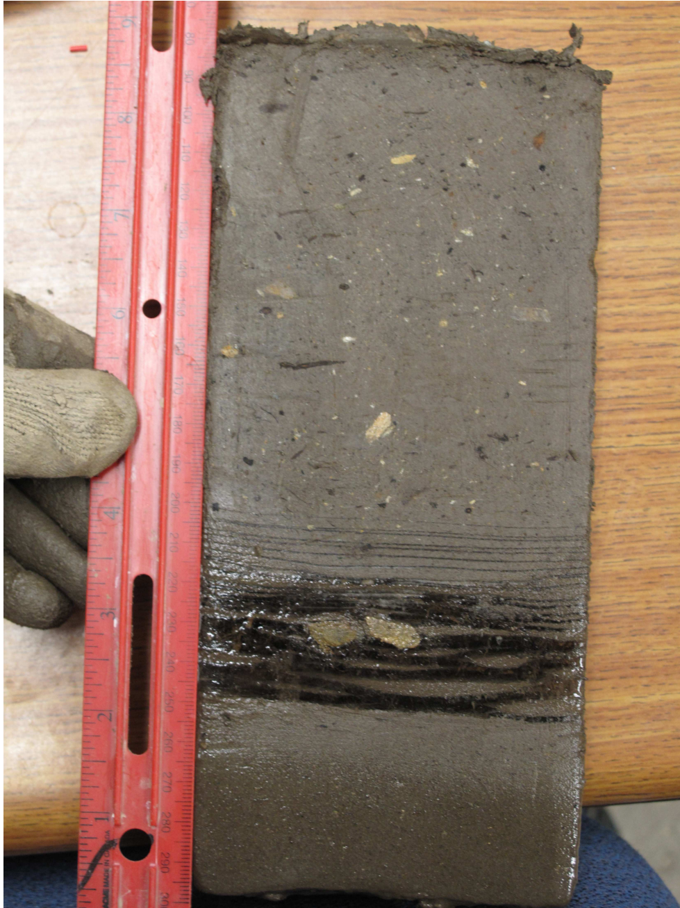
Figure 3.14. Post-frost heave test photograph of vertical section of sample CSI01. Sample was graded due to preparation and saturation process; sample was accidentally inverted during transfer to the Laval Cell (coarse-grained material overlying fine-grained material).
