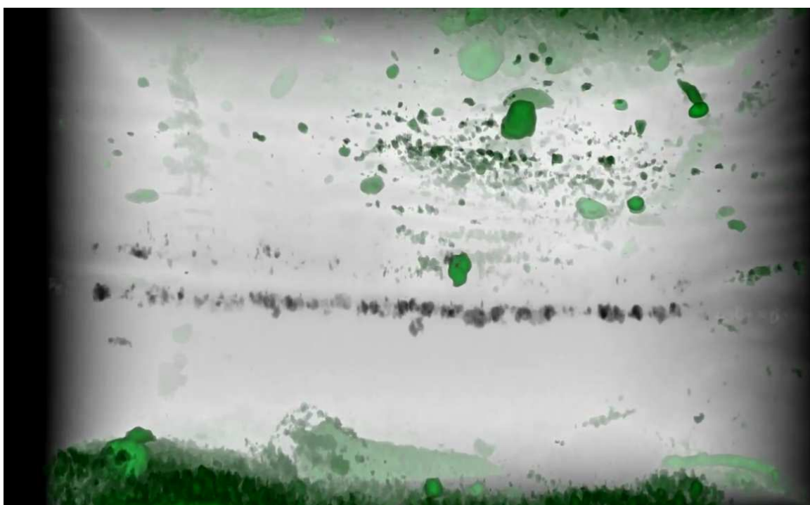
Figure D.2. JSI01 \mu CT rendering video. Video file may be found on attached DVD. Sample is 16.82 mm tall, 24.26 mm wide and deep.
