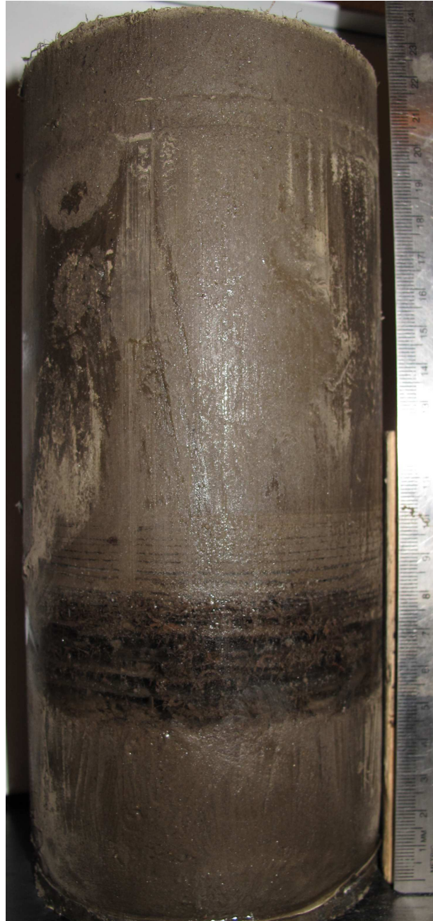
Figure 3.13. Post-frost heave test photograph of sample CSI01.
