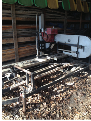
Wood Mizer band saw mill, logs 32" x 16', with sharpening rig
