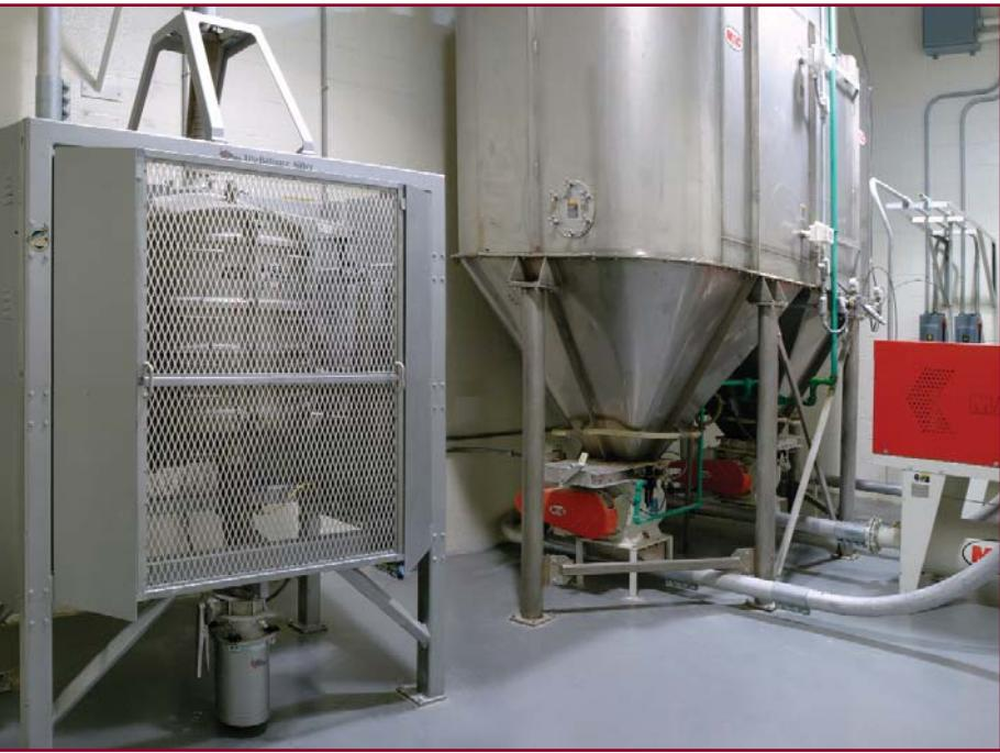
Though in-line sifting was not invented by Great Western, our In-Line sifters are unique. They are **sifters engineered to work under pressure rather than a pressure vessel adapted to act like a sifter**. Because Great Western put the priority in sifting, our In-Line sifters incorporate the features engineers, sanitarians, maintenance personnel and operators have come to expect in any reliable gravity flow sifter.
