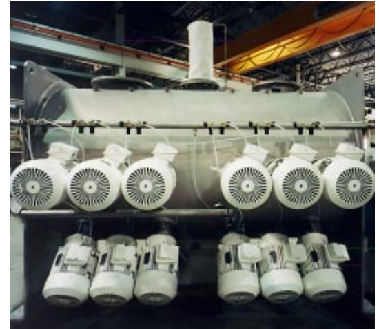
Twelve high speed choppers on this Plow Blender achieve high shear and maximum dispersion.
