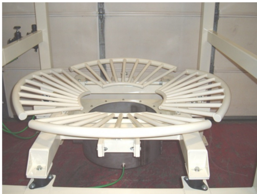
Unique bag bottom support is sanitary and enhances bag discharge properties (with optional pneumatic actuators)
