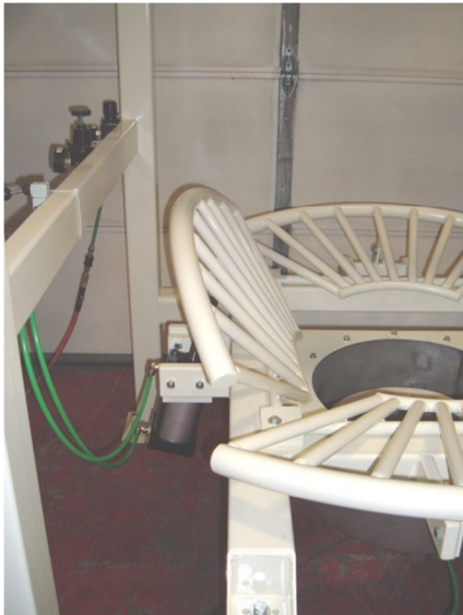
4-section bag support pan hinges to facilitate complete bag discharge
