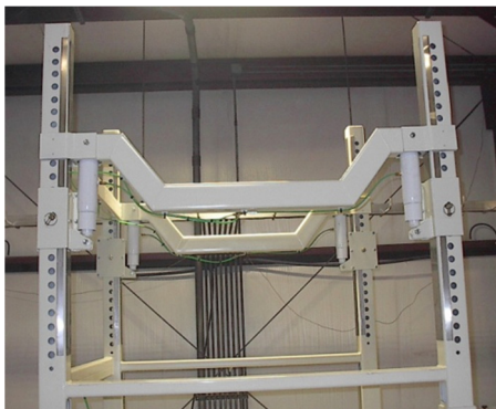
Optional bag lift/stretch assemblies can be added to assist in bag discharge
