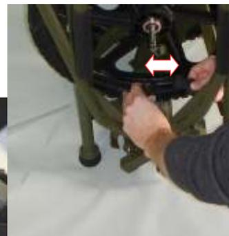
2.) Raise the handles into their operating position. This is done with two motions; first by pulling it away from the carrier, and second by rotating it upward. Each handle will lock in place once it's parallel to the floor.
