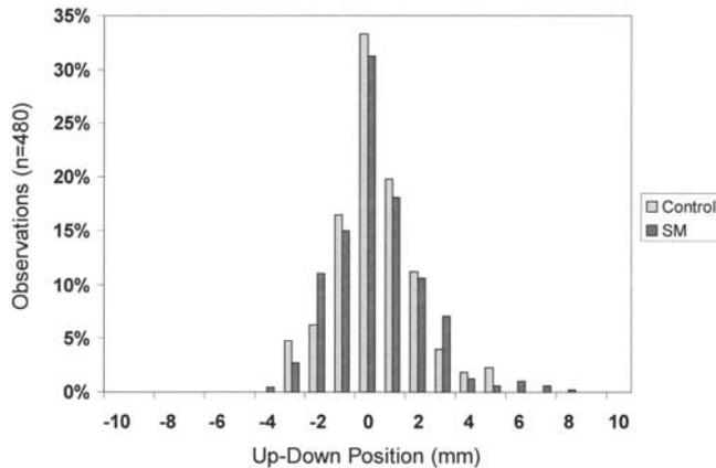
**Fig 3.** Histogram demonstrating normative distribution of up-down position data (mm) recorded while maintaining desired location of TMS coil for both control and SM data sets. Figure contains summary of all values measured for all time conditions ( $N = 480$ ). Similar normative characteristics were returned for left-right and in-out component measures.
