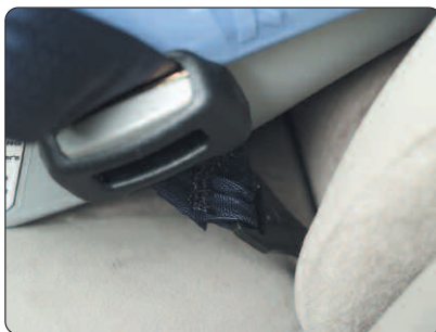
Flexible LATCH hook using anchor bar
