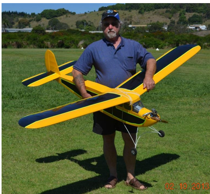
Gary Henderson-Smith proudly displays his Cloud King, 84" span and powered by an Enya 46 four stroke motor.
