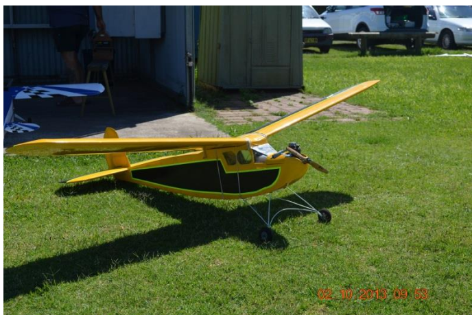
Gary Henderson-Smith proudly displays his Cloud King, 84" span and powered by an Enya 46 four stroke motor.
