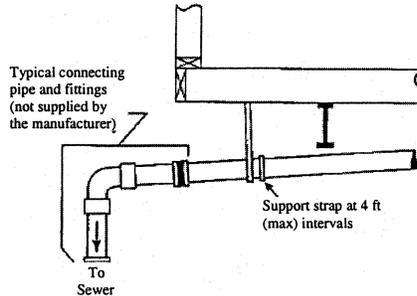
NOTE: Fittings in the drainage system that are subject to freezing, such as P-traps in the floor, are protected with insulation by the manufacturer. Insulation must be replaced if it is removed for access to the P-trap.
