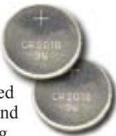
1. Use a toothpick, or other non-conductive probe, to push the old batteries out of the holder.
