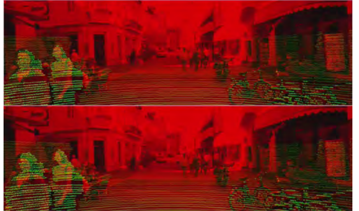
Fig. 10. A frame from the KITTI dataset with velodyne data overlaid in green. Optimized calibration on top, ground truth on bottom. Note the slight misalignment of the faces of the people on the left
