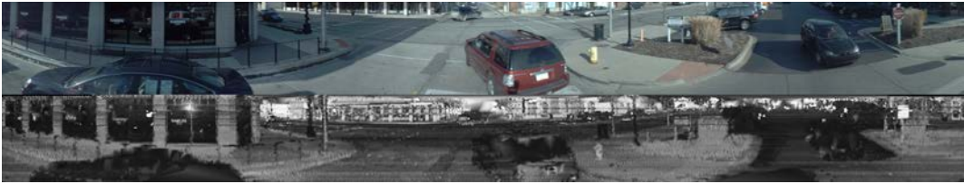
Figure 13: Overlapping region of camera image (top) and lidar scan (bottom) for a typical scan-image pair in the Ford Dataset. The lidar image is coloured by intensity of laser return
