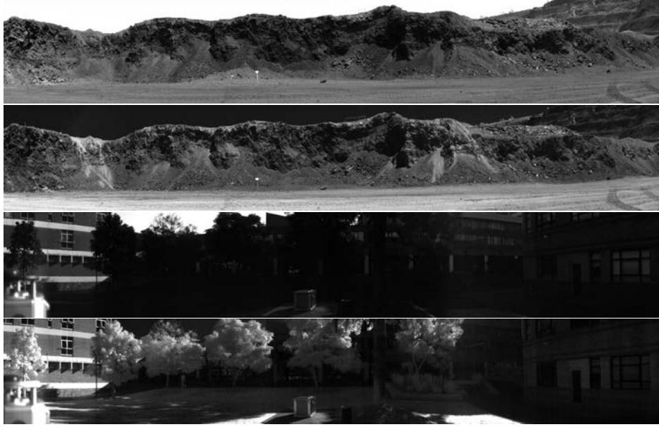
Figure 12: Images captured by hyper-spectral camera. From top to bottom: 420nm mine 1, 950nm mine 1, 420nm ACFR 1, 950nm ACFR 2
