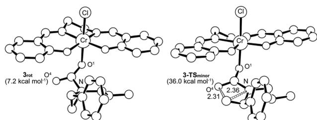
Fig. 7 The transition state structure **3-TS<sub>minor</sub>** (right) for the formation of 4-substituted oxazolidinone, obtained through an asynchronous, concerted pathway from the corresponding intermediate **3<sub>rot</sub>** (left). The “lengths” for the relevant C–N and C–O bonds (in Å) are indicated on the structure. For clarity, all hydrogens have been removed.
