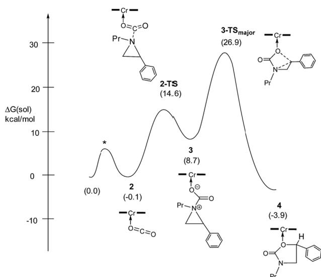
Fig. 5 The complete free-energy profile for the formation of the major 5-substituted oxazolidinone product from the (salen)Cr<sup>III</sup>Cl-catalyzed [aziridine + CO<sub>2</sub>] coupling in the absence of DMAP cocatalyst. All energy values have been solvation-corrected. The TS marked as \* was not located computationally and is only shown for illustrative purposes.
