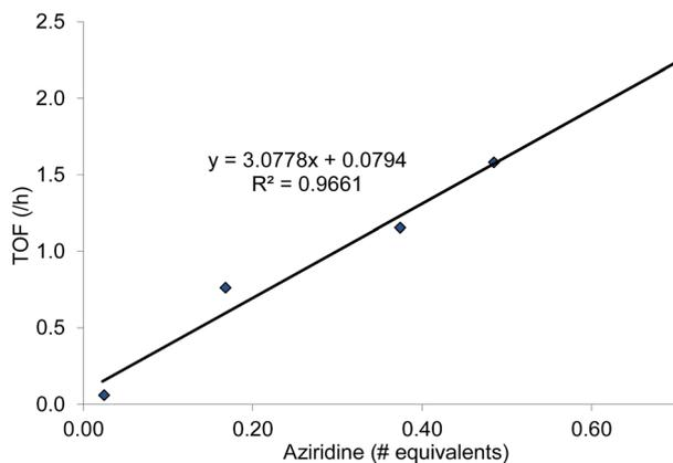
Fig. 12 Kinetic plots of the coupling reaction between *N*-propyl-2-phenylaziridine and CO<sub>2</sub> catalyzed by (salen)Cr<sup>III</sup>Cl. General reaction conditions: *N*-*n*-propyl-2-phenylaziridine (varying amounts, between 0.088 g and 0.228 g; 0.55 mmol to 1.42 mmol), catalyst (5.8 mg, 0.01 mmol), 400 psig CO<sub>2</sub>, CH<sub>2</sub>Cl<sub>2</sub> (1.8 mL), rt, 24 h. Top: in the absence of DMAP cocatalyst. Bottom: in the presence of 2 equiv. of DMAP cocatalyst (2.45 mg, 0.02 mmol).
